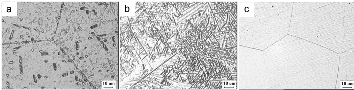
Fig. 1. Microstructure of the Ti–12Mo–5Zr alloys: (a) homogenized; (b) 1053 K ST; and (c) 1133 K ST.
